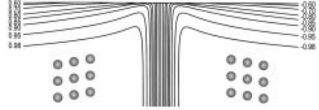
Fig. 2. Distribution of the order parameter Q at the surface of the lattice (first 50 layers). Lines represent constant Q/Q_0 . There are three lines in the middle of the twin domain wall that are not labeled, they represent the Q/Q_0 values of 0.40, 0.00, and -0.40 respectively. Notice the steepness of the gradient of Q/Q_0 through the twin domain wall. The two structures represent sheared twin atomic configurations in the bulk (far from the twin domain wall and surfaces).
